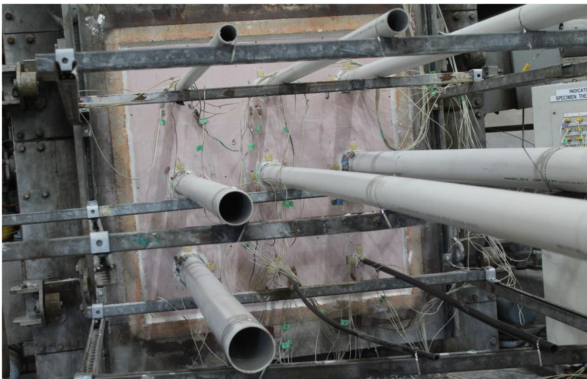
Figure 13 – Unexposed face prior to test commencement
